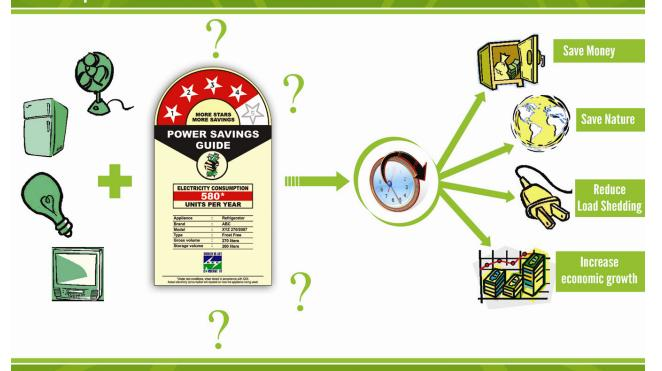
**Energy-efficiency labels** are informative labels affixed to manufactured products to describe the product's energy performance (usually in the form of energy use, efficiency, or energy cost); these labels give consumers the data necessary to make informed purchases.
